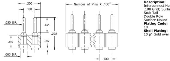
Jescription: Interconnect Header .100 Grid; Surface Mount Pin Header Stub Tail Double Row Surface Mount Plating Code: 10 Shell Plating: 10 μ" Gold over 100 μ" Nickel
